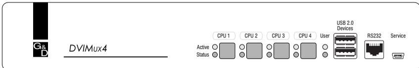
**Figure 1: Front view of the KVM switch**
