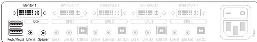
**Figure 2: Interfaces to connect the console devices**
