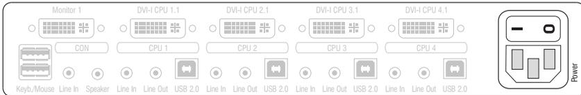
**Figure 4: Interface to connect the power supply**
