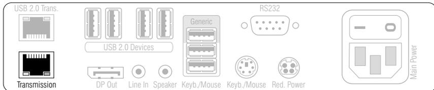
**Transmission:** Plug a category 5e (or better) twisted pair cable, which is available as accessory, into this interface. Connect the other end of the cable to the respective interface of the computer module or to one of the *Dynamic Ports* of a compatible matrix (see page 5).
