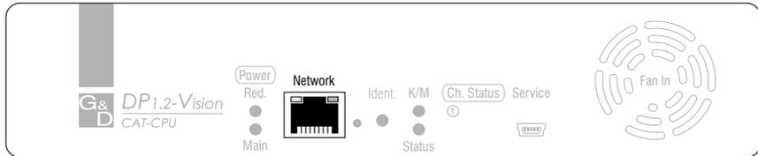
**NOTE:** If desired, connect the network interface to a local network. This enables you to access the **Config Panel** web application from this network and to send syslog messages to this network.
