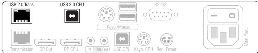
**USB 2.0 CPU:** Use the *USB-AM/BM-2* cable to connect one of the computer's USB interfaces to this interface.
