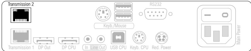
**Transmission 2:** Plug a category 5e (or better) twisted pair cable, which is available as accessory, into this interface. Connect the other end of the cable to the respective interface of a compatible computer module or matrix switch.
